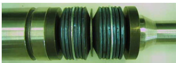
Fig. 12 Washer configuration for test F
