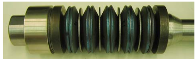
Fig. 8 Washer configuration for test D
